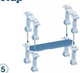
• Fit two more bridge supports onto the bridge assembly, as shown.
